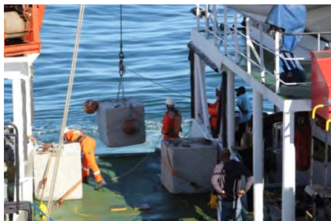
Figure 23: DEA: O&C dive team aboard DEA's research vessel Algoa deploying moorings for the research buoys to be attached (SHBML, November 2017)
