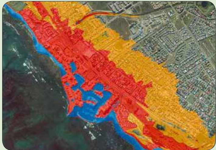
Figure 9: Projected areas of the Cape Town foreshore inundated under different climate change scenarios.
