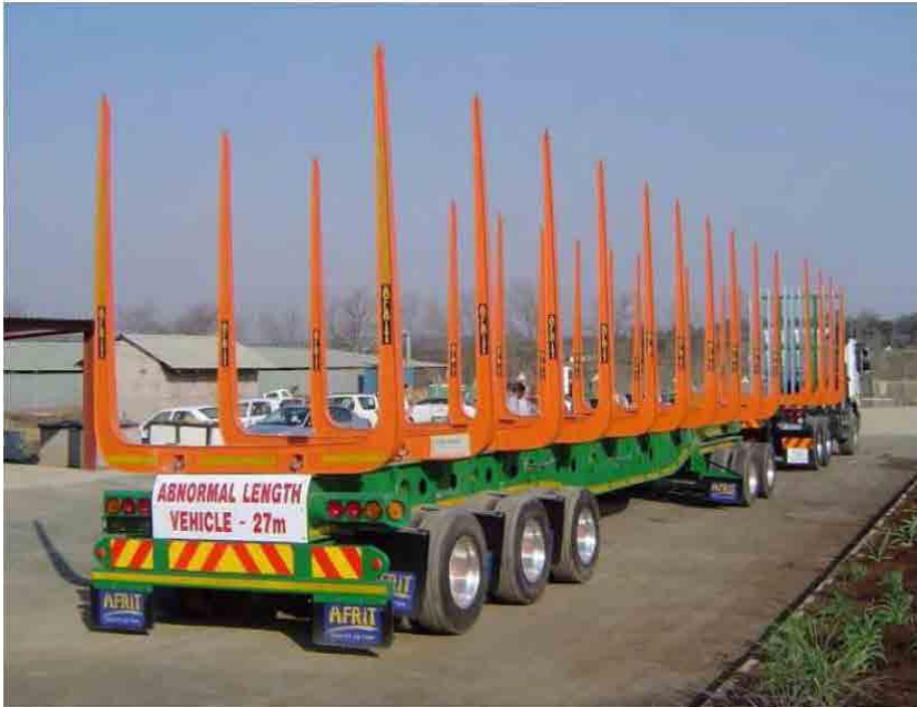
Figure 5-14: Example of the PBS Vehicles used by Sappi (overall length of 27.0m and maximum combination mass of 67.5 tonnes)
