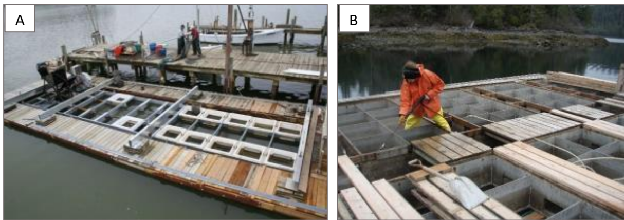
FIGURE 24: EXAMPLES OF LAND-BASED NURSERY UPWELLING SYSTEMS (SOURCE: BLUE STAR OYSTER CO., 2016).
