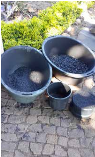
(ii) Fine-grained biochar (following a process of grinding to different-sized grains for different uses).
