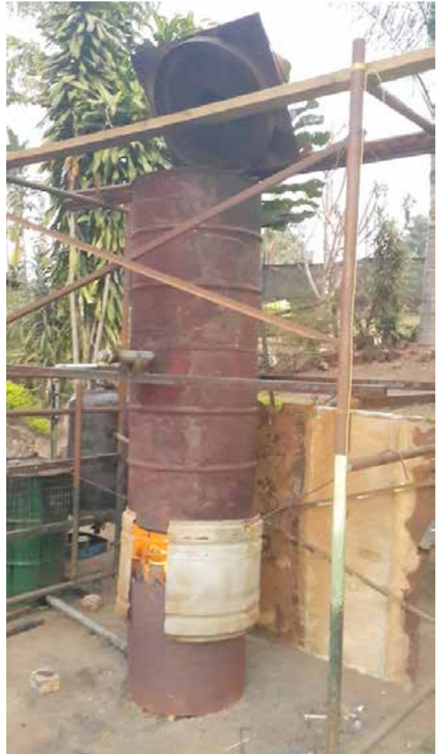
(ii) A vertical burner at the Sustainable People's Project. Gas from the top of the burner is recycled to the combustion zone as an additional fuel. This unit is configured to recover the bio-oil shown in Figure 4(i).
