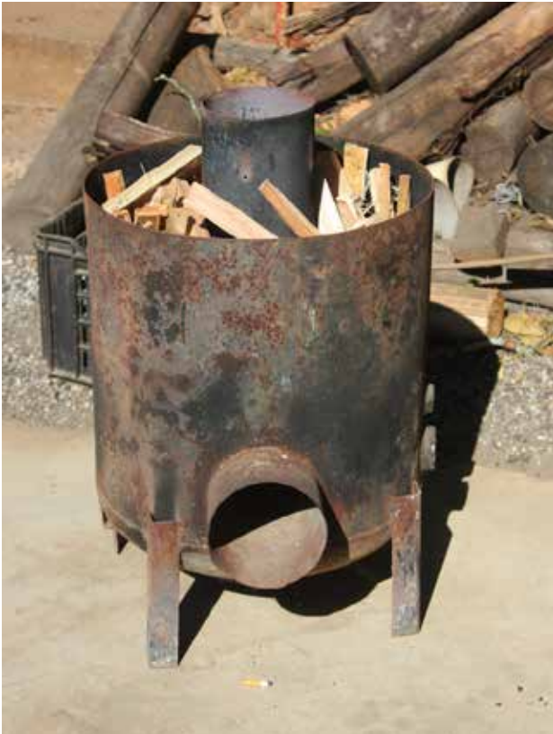
(i) A basic burner at the Sustainable People's Project in Tzaneen. This device can be used as a stove, while at the same time producing biochar.
