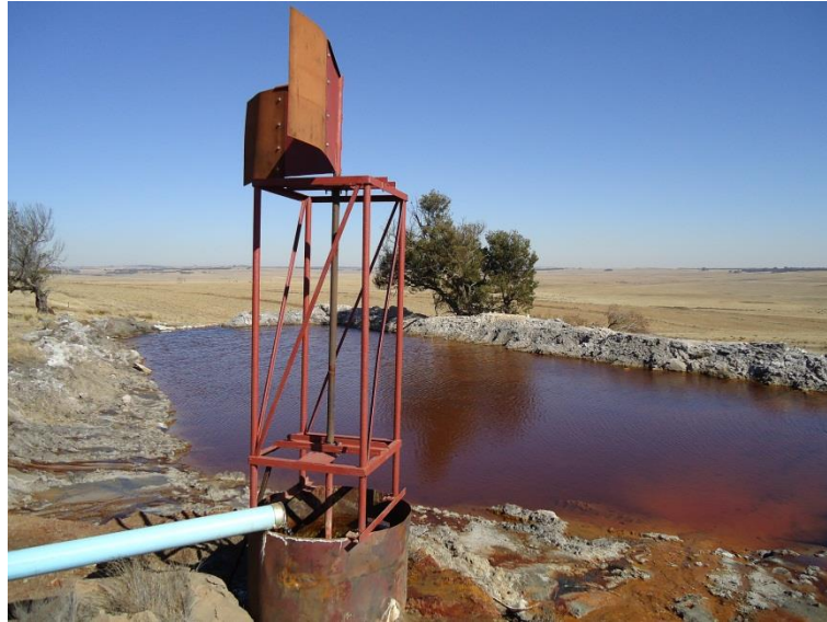
Figure 3. Novel passive treatment system installed at a coal mine discharge point in Mpumalanga. This device aims to agitate a lime-AMD slurry using a vertical-axis wind turbine. At the time that this photograph was taken, the system was not functioning due to the breakage of the turbine.
