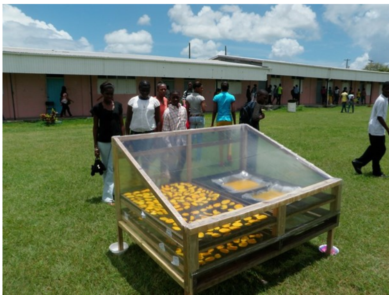
Figure 9.1: A simple solar dryer for home use.
