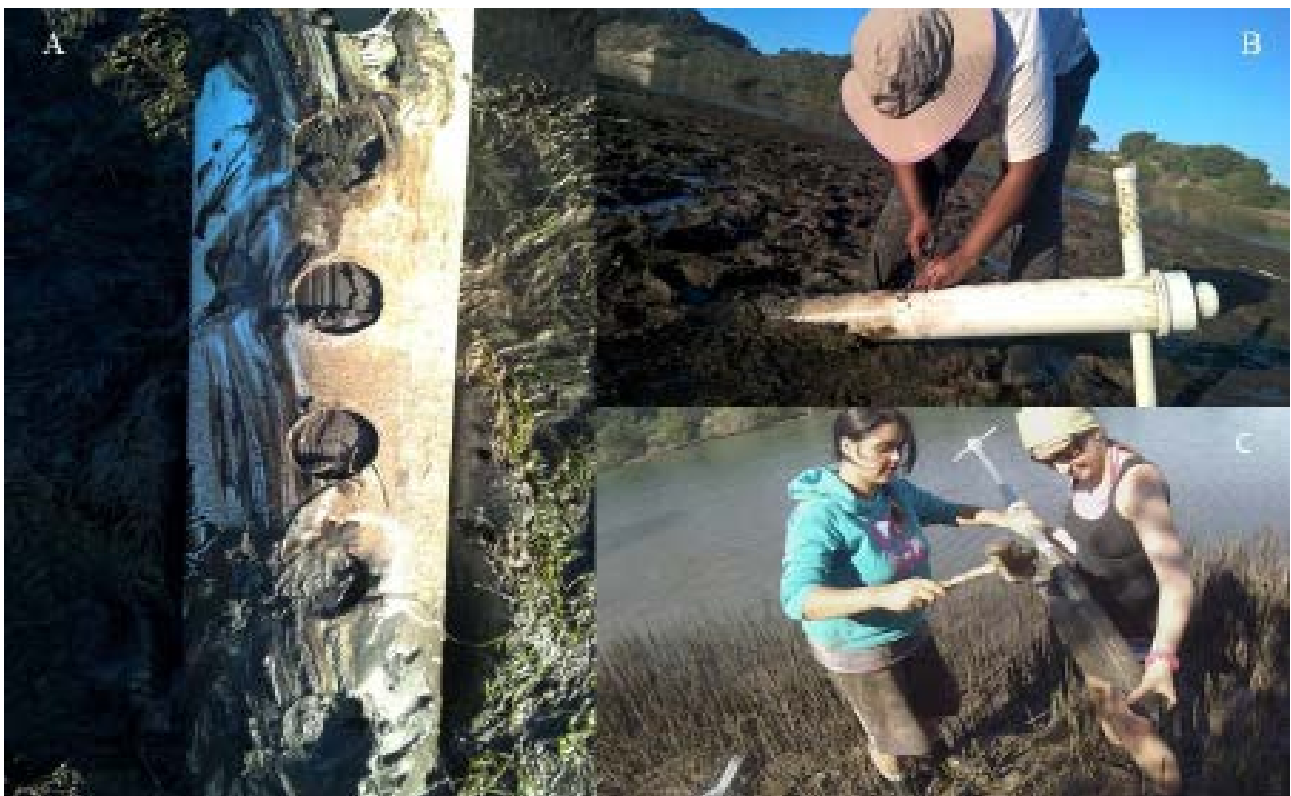
FIGURE 1.5: FIELD SAMPLING FOR SOIL CORES AT THE NXAXO ESTUARY. A PVC PIPE CORER WITH PRE-DRILLED HOLES (A) WAS USED IN SALT MARSH AND SEAGRASS AND A SYRINGE WAS USED TO EXTRACT THE SUBSAMPLES (B). A RUSSIAN PEAT CORER WAS USED IN THE MANGROVES (C). FIGURE ADAPTED FROM BANDA ET AL. (2021).
