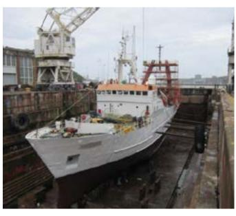
Dry dock: RV Algoa undergoing servicing and maintenance in the dry dock
