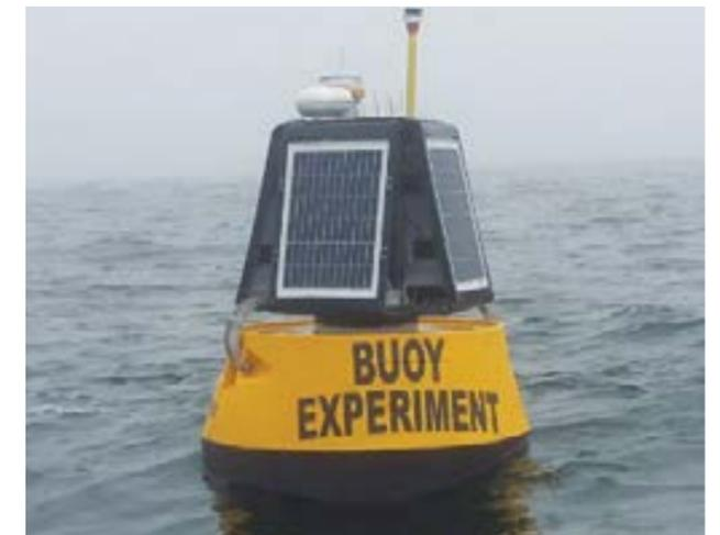
Data Buoy monitoring surface and bottom water parameters (fluorescence, temperature, oxygen, salinity, currents) and atmospheric weather
