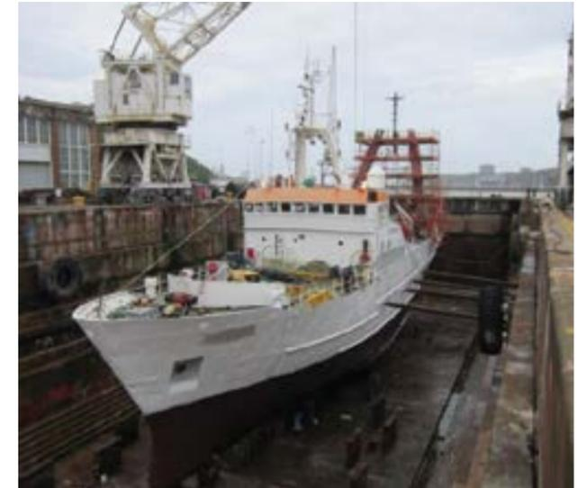
Dry dock: RV *Algoa* undergoing servicing and maintenance in the dry dock
