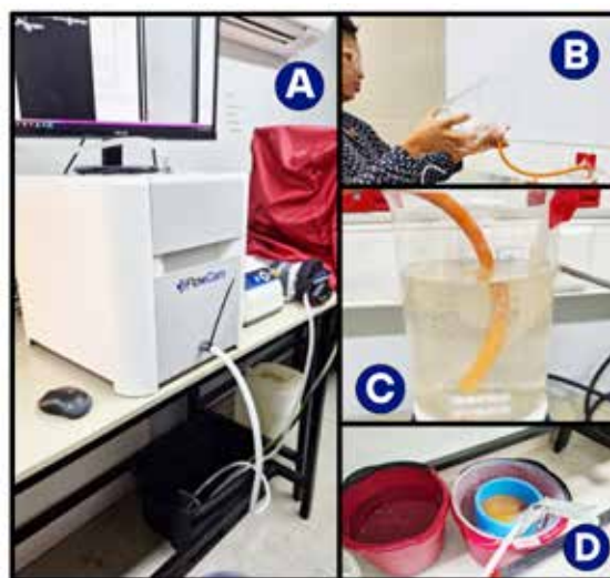
Figure 2. (A) Modified setup of the FlowCam Macro, (B) and (C) re-filling the beaker to minimise air bubbles, and (D) retention of the sample by separation of animals and water at the outlet.
