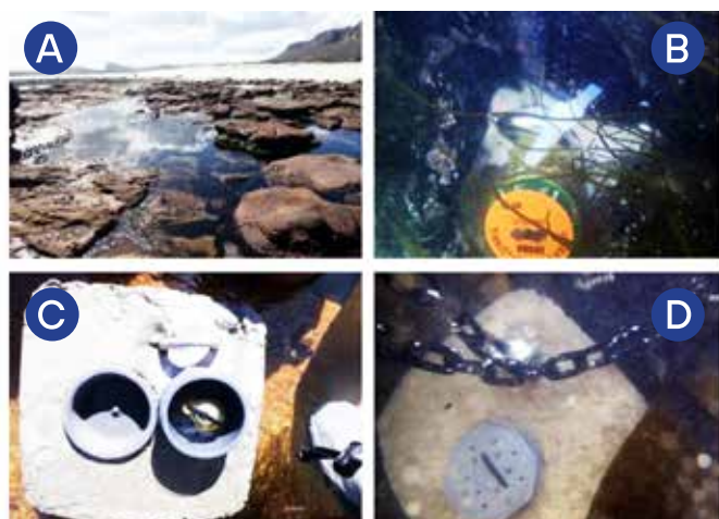
Figure 1. In intertidal rock pools (A), temperature loggers are attached via a cable tie to either an ibolt drilled into the rock (B) or housed inside a mooring block (C–D).
