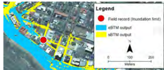
Figure 2. Locations of field recording (red point) and results from the simple Bathtub Model (sBTM, yellow) overlaid with the enhanced Bathtub Model (eBTM, blue), using digital surface models (DSMs).
