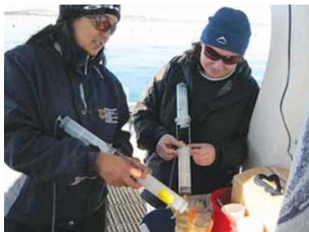
Figure 35: Filtering of effluent water.
