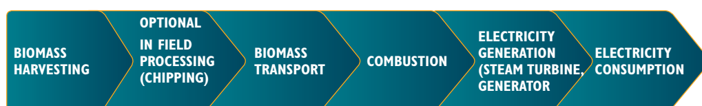
Figure 10.8: Biomass to energy process (electricity)
