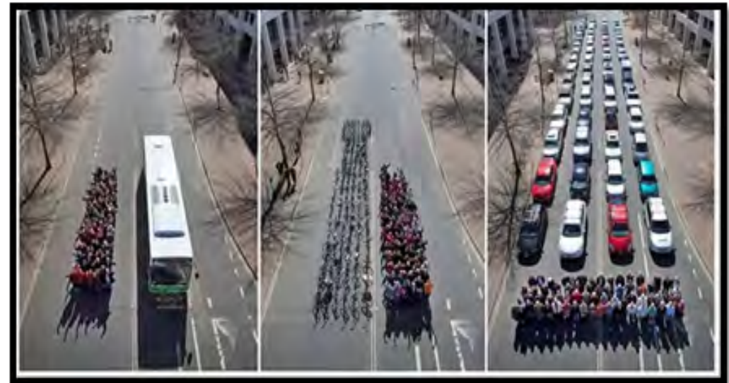
Figure 2.2 Comparison of space used to transport the same number of people by bus, bicycle and car. Source: www.shoroc.com
