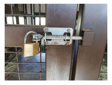
Locking bar with a spring and padlock for every door and gate.
