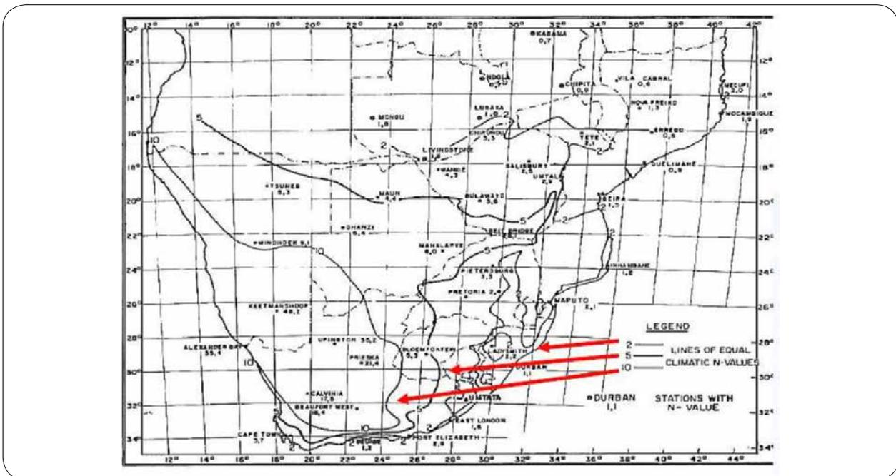
Figure 52: Classification of climatic regions for the selection of pavement binder type (Weinert 1980)
