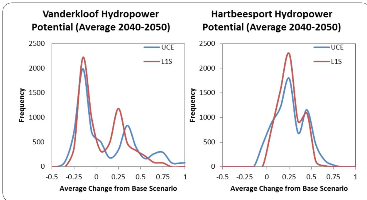
Figure 39: Hybrid frequency distribution (HFD) of the change in the potential average annual hydropower production for the Vanderkloof and Hartbeespoort dams for the UCE and LIS climate scenarios.
