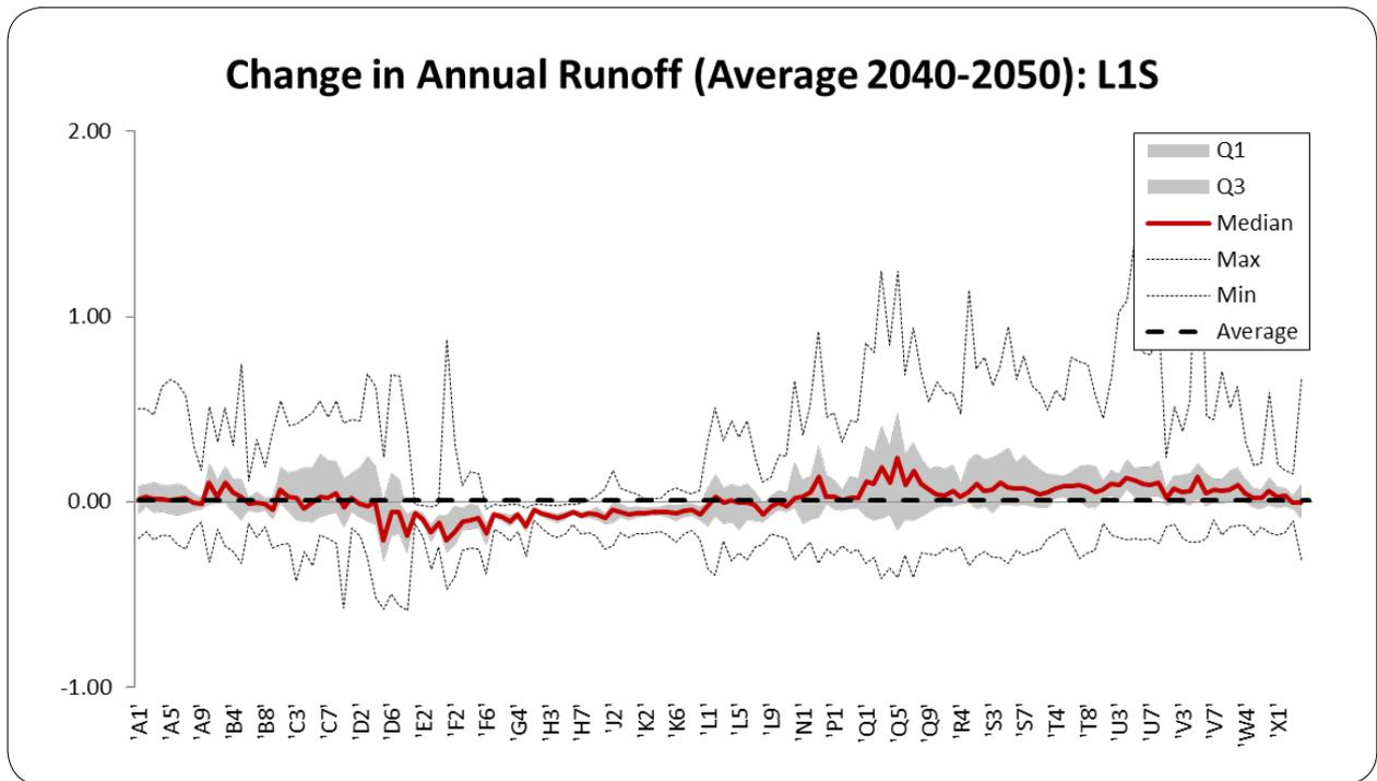
Figure 26: Range of potential impacts of climate change on the average annual catchment runoff for all secondary catchments for the period 2040–2050 due to the LIS scenario relative to the base scenario.
