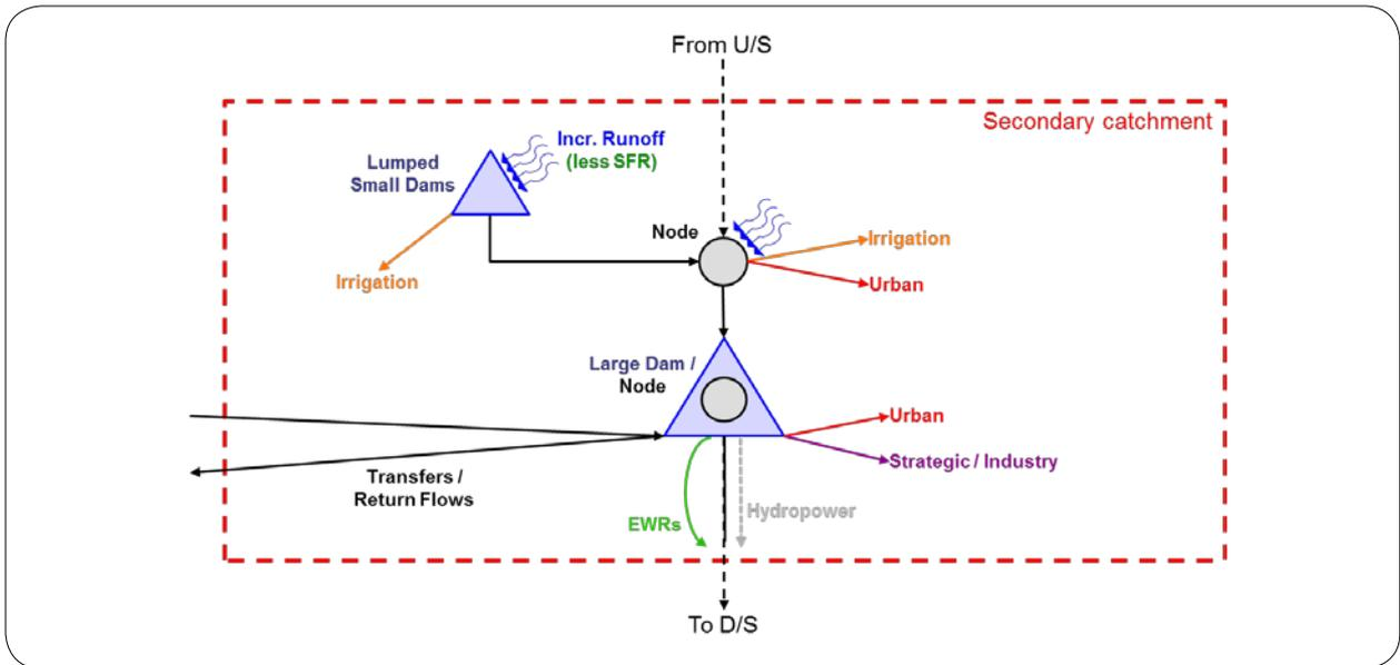
Figure 4: Generic modelling unit used for configuration of the WRYM
