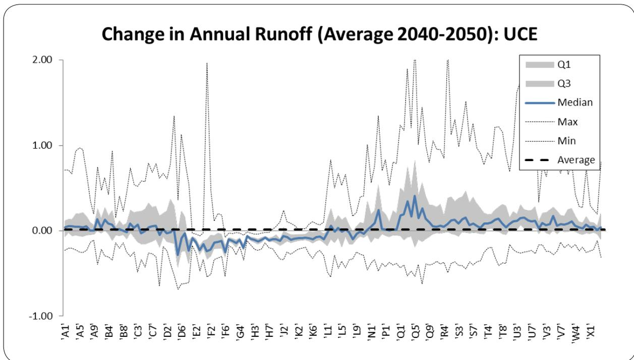
Figure 25: Range of potential impacts of climate change on the average annual catchment runoff for all secondary catchments for the period 2040–2050 due to the UCE scenario relative to the base scenario.
