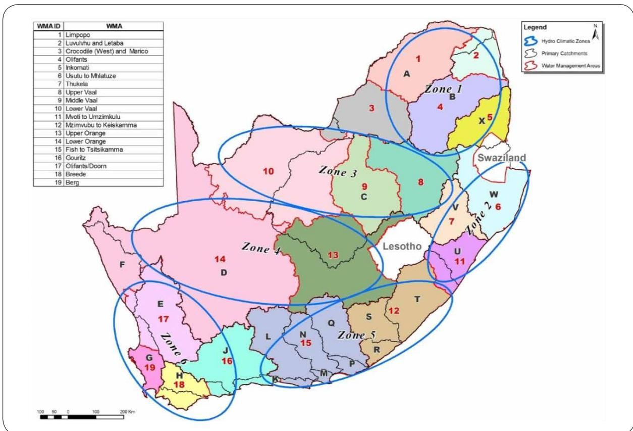
Figure 6: Map of South Africa showing the name and location of the nineteen water management areas, primary catchments and the grouping of catchments into six general hydro-climatic zones.
