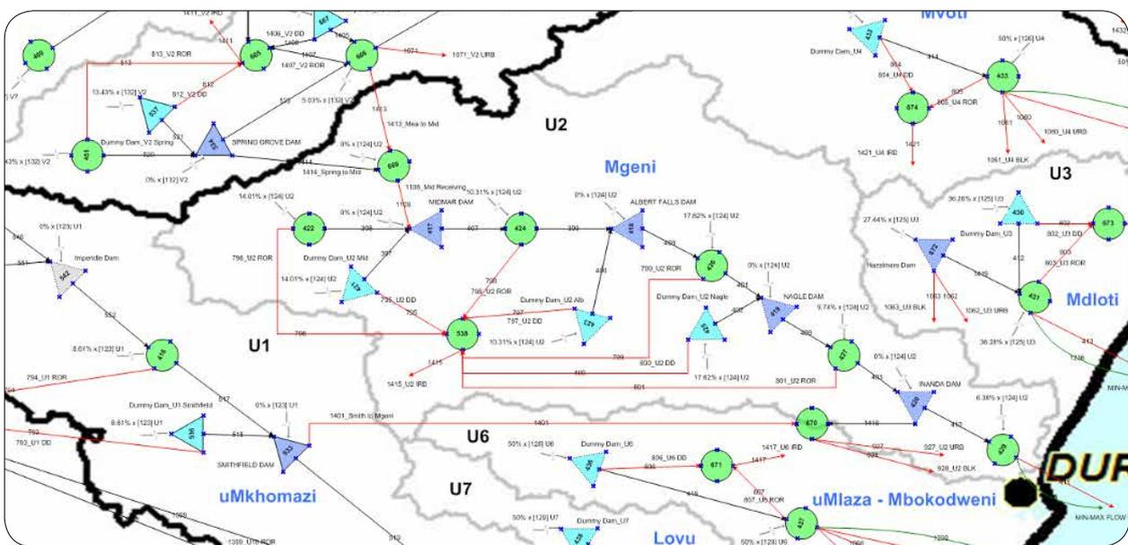
Figure 4: Details of a portion of the national WRYM system model (Mooi-Mgeni River System) (Drawn by authors)
