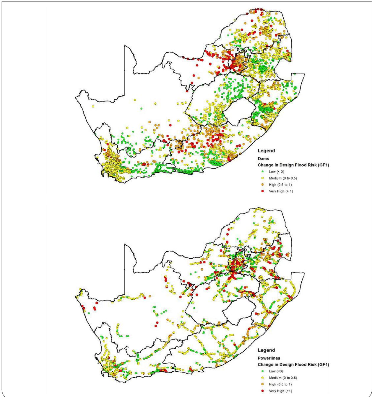
Figure 17: Frequency distributions of extreme potential impacts on the design flood (1:100 year) for key infrastructure under four climate change models (top, left) and the relative risk for individual structures for the climate model with the greatest general impact up to 2100 (GF1). (Analysis based on potential changes in 1:100 year RI flood – no consideration of hydraulic characteristics of individual structures.)
