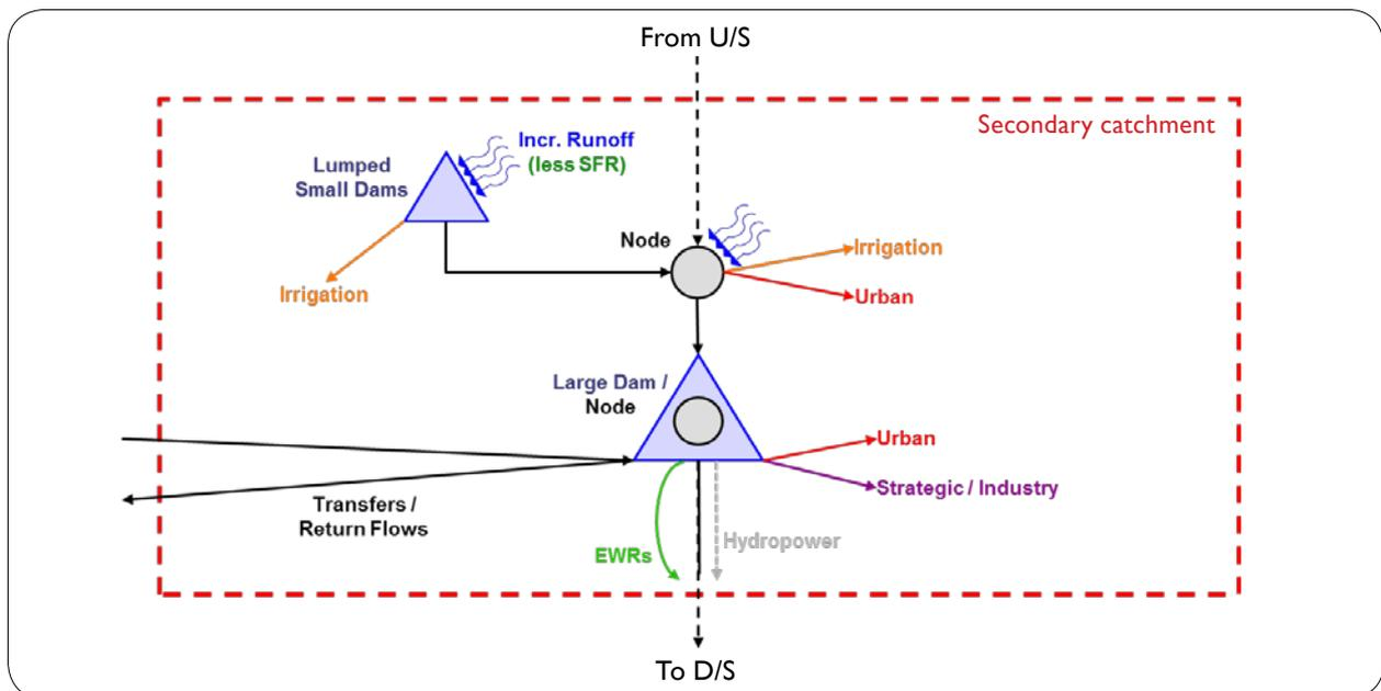
Figure 2: Generic modelling unit used for configuring the WRYM (Drawn by authors)
