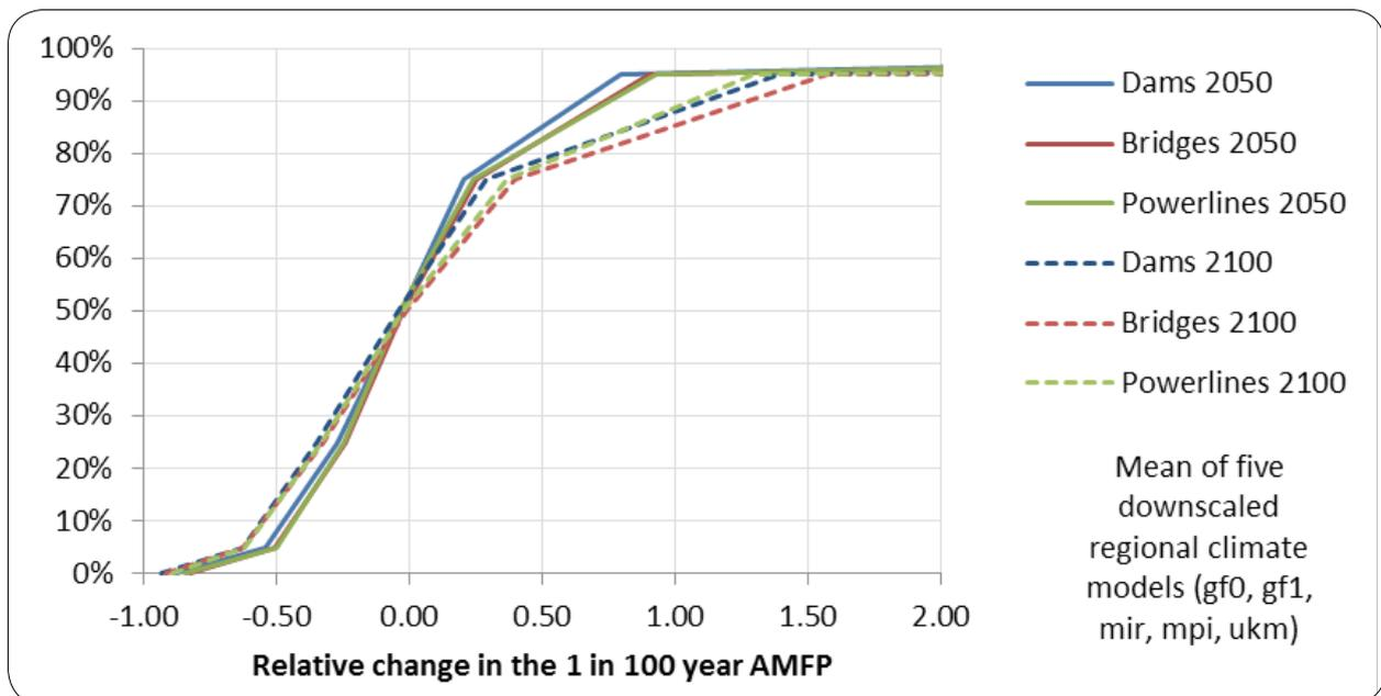
Figure 16: Cumulative frequency distributions of the relative changes in the 1 in 100 year annual maximum flood peak (AMFP) key infrastructure across South Africa by 2050 and 2100 compared to the historical period (representing the average impacts of five climate models). (Authors' compilation)
