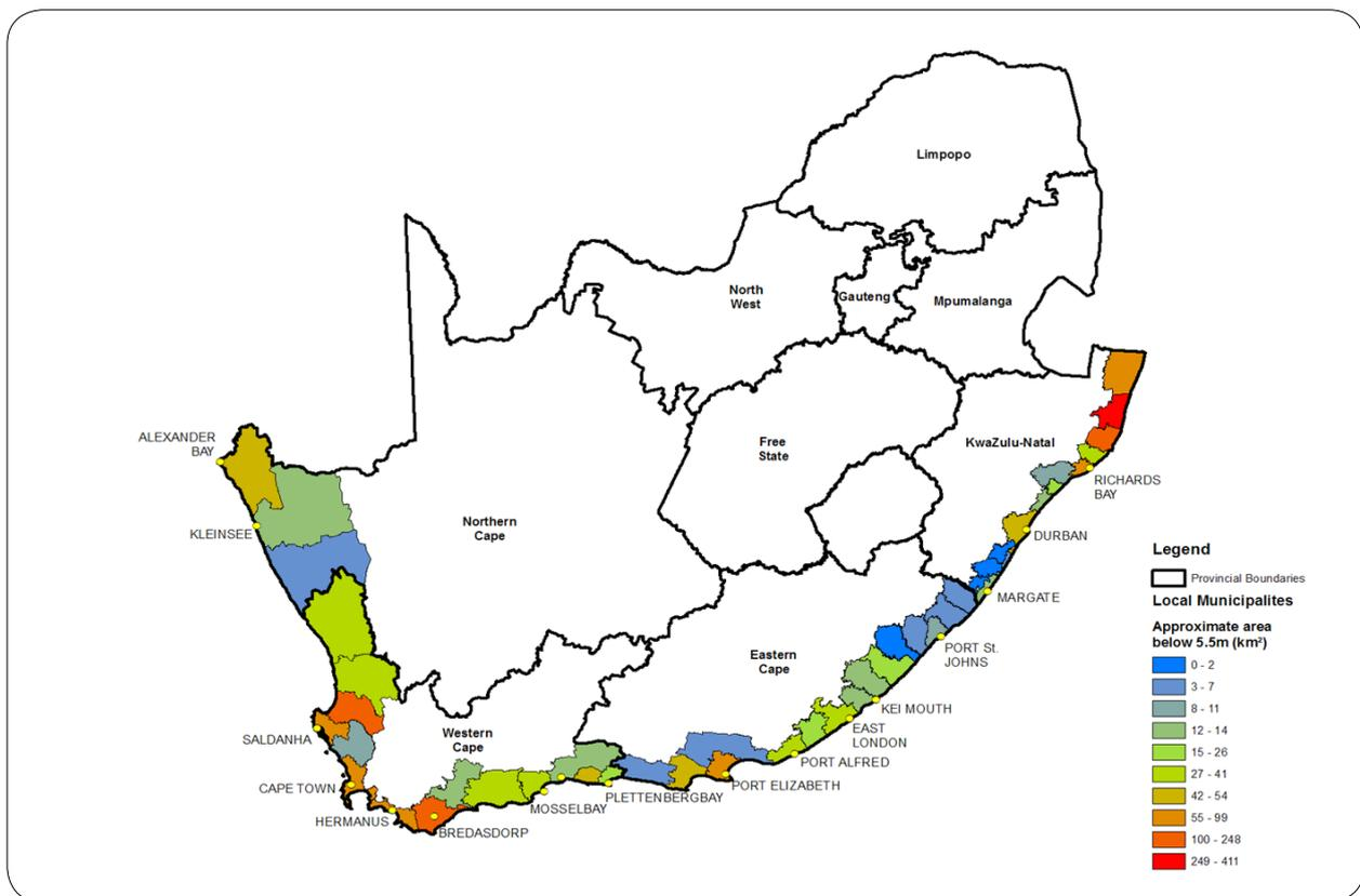
Figure 21: Approximate area of coastal local municipalities below 5.5m elevation above current mean sea level (MSL).
