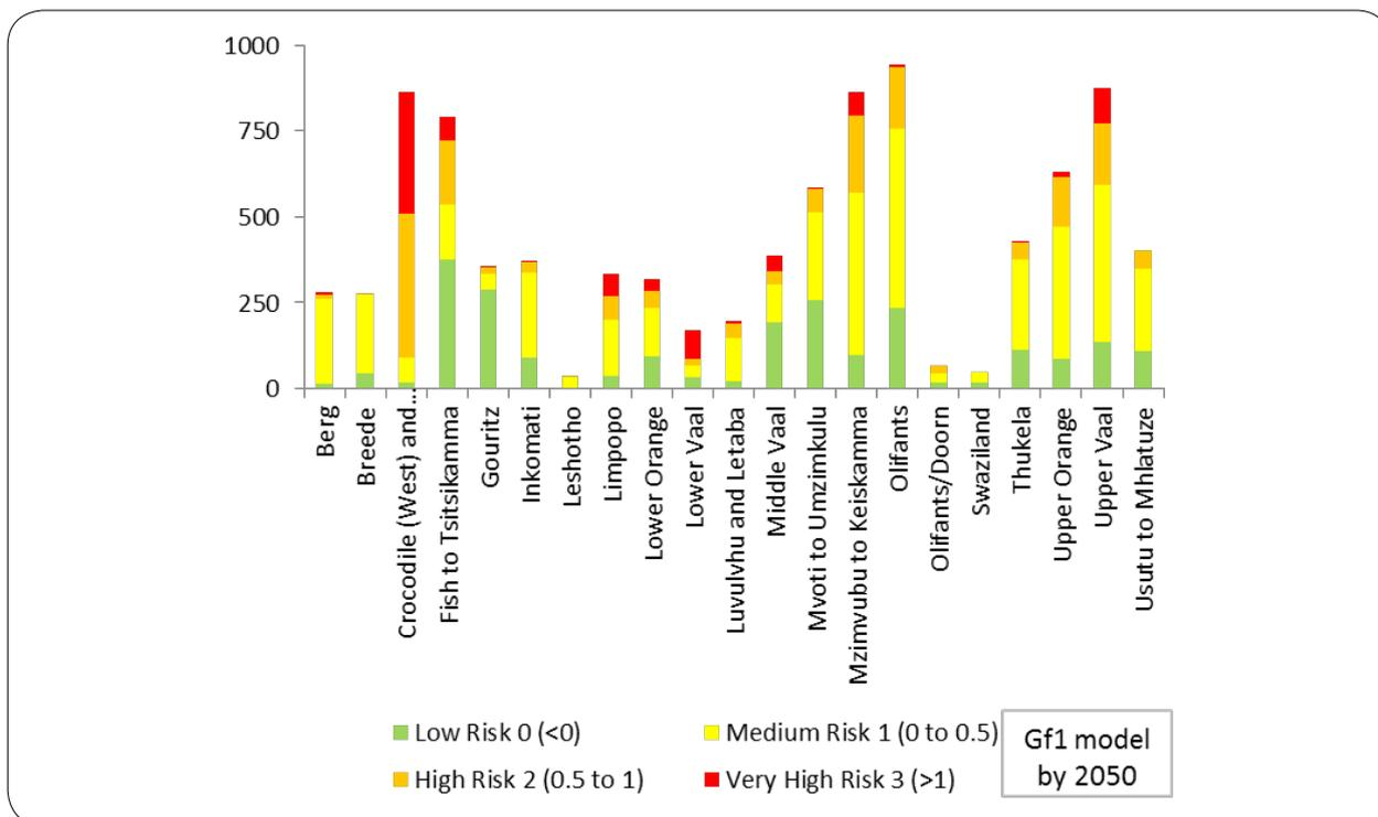
Figure 18: Number of bridges in each WMA in each risk class defined in terms of the maximum relative increase in the 1:100 year design flood by 2050 for the GFI climate model.
