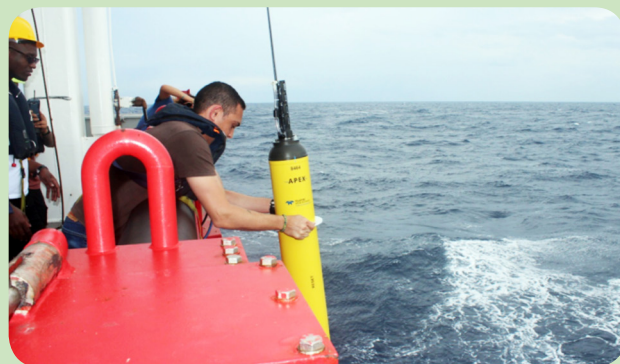
Above: DEA's researcher deploys the Argo float which measures ocean temperature, salinity and oxygen while drifting with Oceanic Currents.
