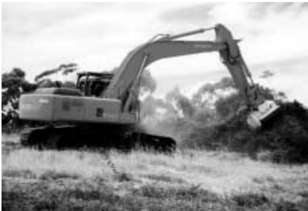
Earth moving equipment fitted with a grooming head treating a dense stand of blackberry.
