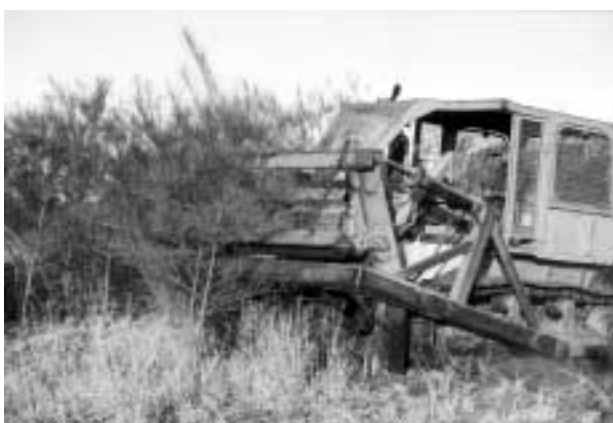
Mechanical control of parkinsonia ( Parkinsonia aculeata ) with an Ellrott front-mounted bladeplough. Photo: John McKenzie
