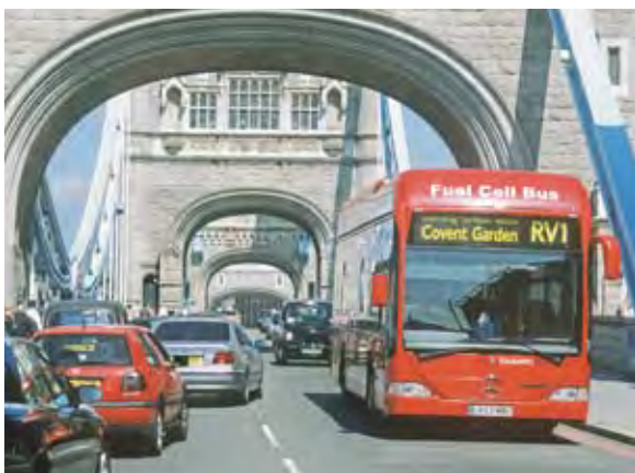
© Martin Bond / Still Pictures A hydrogen fuel cell-powered electric bus in service crossing Tower Bridge in London. Part of the Clean Urban Transport Europe (CUTE) demonstration project testing 27 such pollution-free buses in nine European cities.
