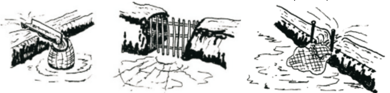
Variety of screens placed at pond inlets: basket, sticks and mesh bag.
