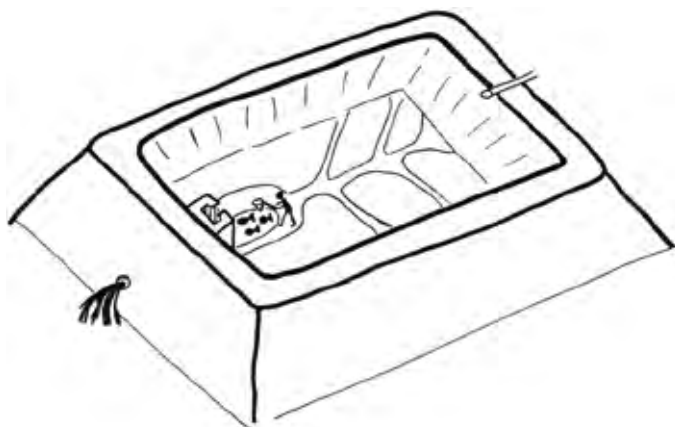
A channel through the middle of the pond can help with draining the pond and harvesting fish.
