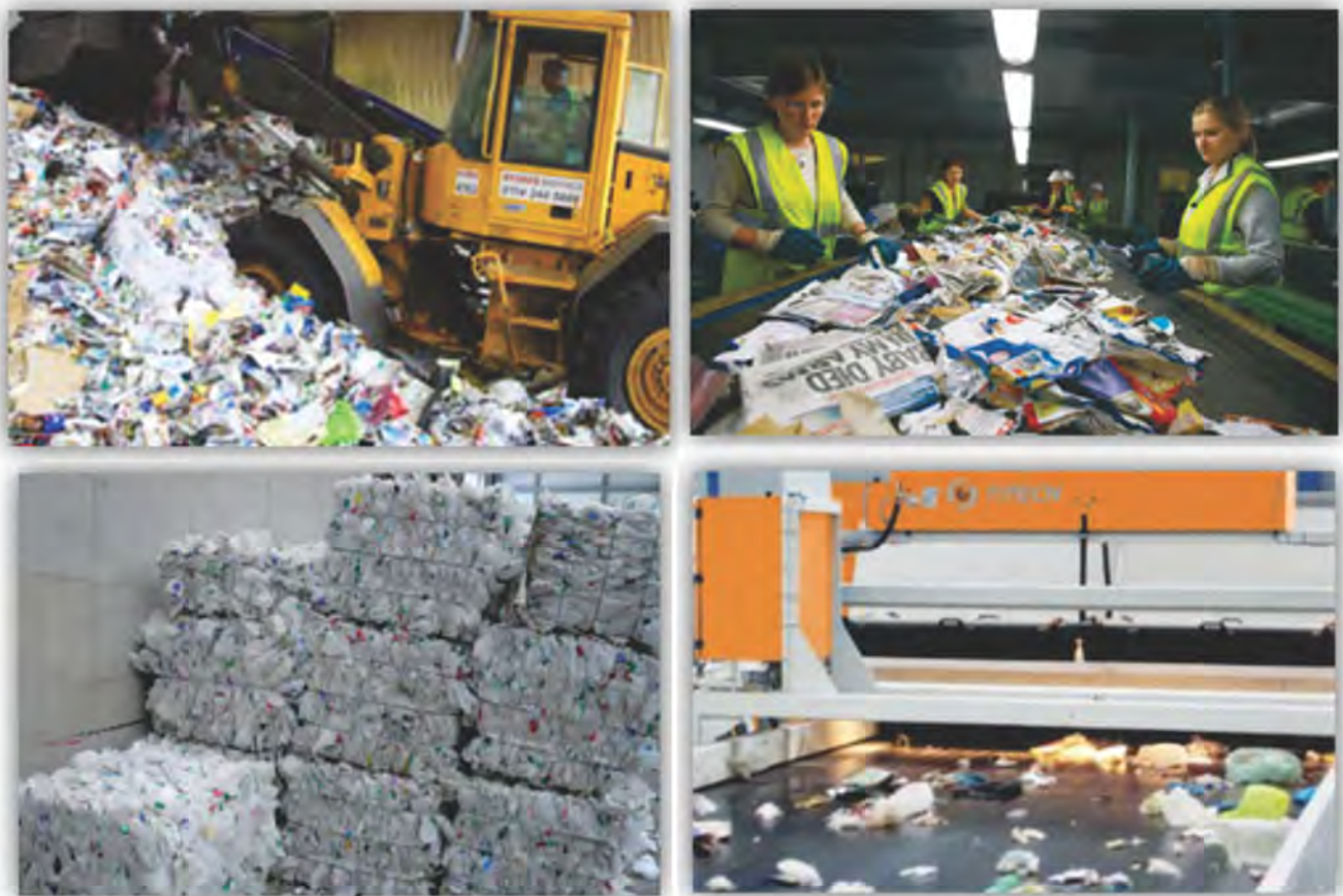
Figure 9: (clockwise from top left) Mixed recyclable materials in tipping hall (image courtesy of WRAO); manual picking line (image courtesy of WRAP); mixed plastics approaching a NIR sorting machine (image courtesy of Titech); baled separated HDPE plastic bottles (image courtesy of WRAP)
