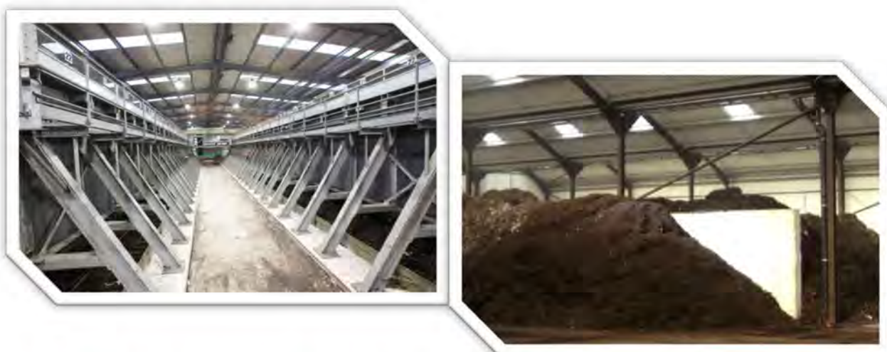
Figure 17: Inside a tunnel method IVC facility (image courtesy of Viridor); IVC compost (image courtesy of Sita)
