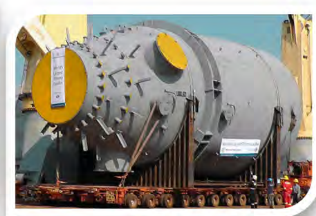
Figure 23: Demonstration plasma torches (image courtesy of AlterNRG); delivery of large (350k tonnes per annum) plasma gasifier in NE England (image courtesy of AlterNRG / Air Products)
