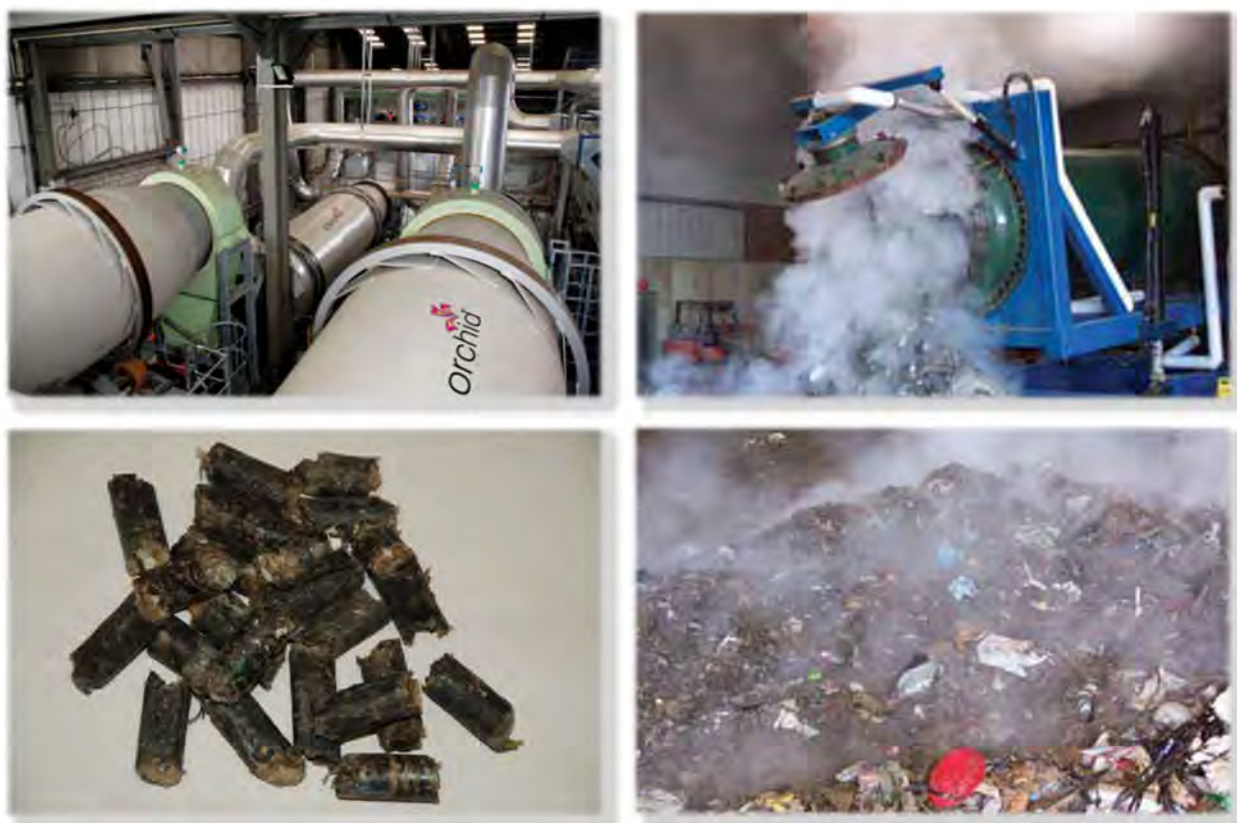
Figure 28: (clockwise from top left) Non-pressurised heat vessels (Orchid Environmental); end of process / emptying of an autoclave vessel; autoclaved waste; pelletised RDF from heat non-pressurised heat vessels (Orchid Environmental)
