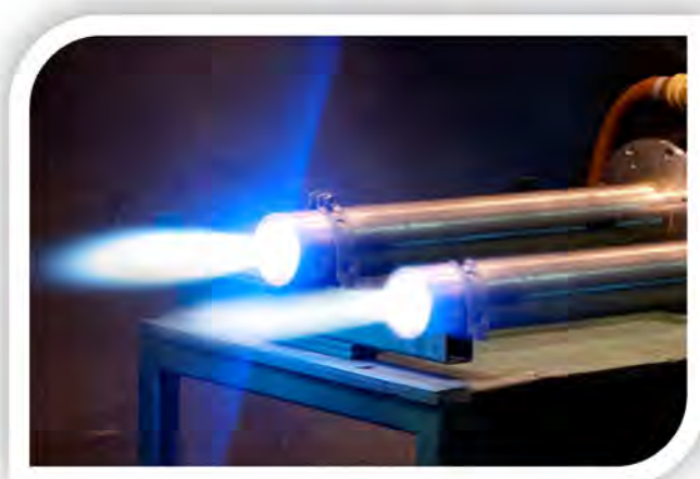
Figure 23: Demonstration plasma torches (image courtesy of AlterNRG); delivery of large (350k tonnes per annum) plasma gasifier in NE England (image courtesy of AlterNRG / Air Products)
