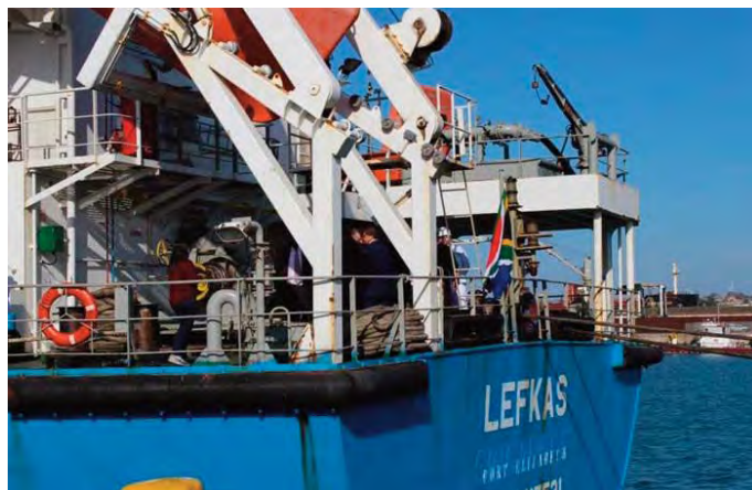
The MT Lefkas is a bunker (ship fuelling) vessel, owned by Greek shipping group Aegean. Recently registered under the South African flag, it will be officially stationed at Port Elizabeth to supply fuel at sea to vessels sailing Africa's southern oceans.
