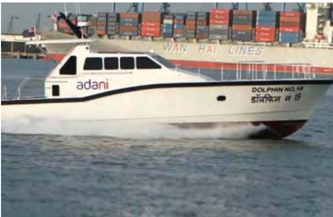
16.7m Patrol boat, designed by Icarus Marine Many vessel builders use proven designs, to be confident that finished products will meet contracted speed requirements. In the absence of a proven design it is common practice to test the hull of the vessel at a ship model test basin. Icarus Marine in Cape Town uses a 100m model test tank at Stellenbosch University, as well as computational fluid dynamics (CFD) analysis, to ensure predictable performance of full-scale, original designs.
