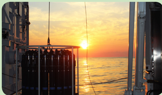
Above: CTD being lowered into Tanzanian waters. The CTD has an oxygen sensor and fluorescence sensor that measures how much chlorophyll is in the water, it can also be used as a measurement of phytoplankton (organisms that produce half of the world's oxygen).
