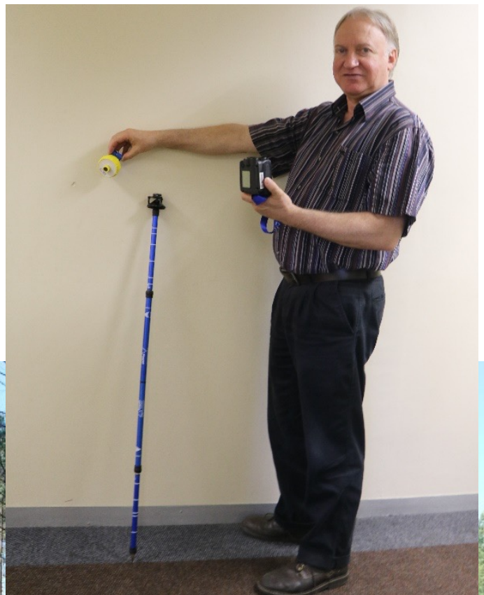
Above: Mr Bester with the Vertex Laser VL402 which allows you to measure, map, process and store forest and field data.
