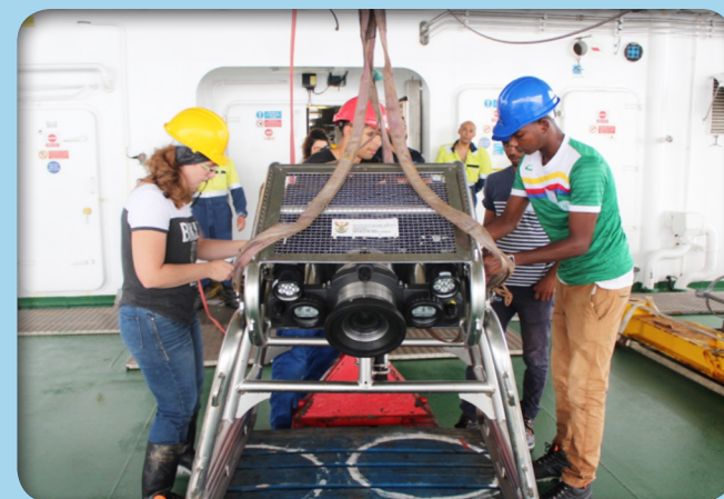
Above: DEFF's benthic camera (ski-monkey) used for underwater observations aboard the SA Agulhas II. (Photo by Tshego Letshwiti)
