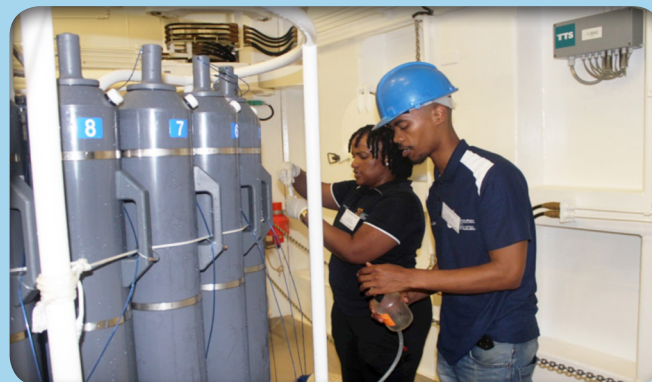
Above: Samples of dissolved oxygen, dissolved alkalinity, nutrients and chlorophyll being taken from the Conductivity Temperature Depth (CTD) device. (Photo by Tshego Letshwiti)
