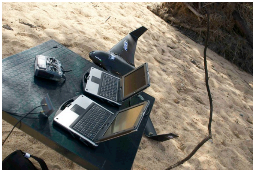
A basic ground station setup: Off the shelf versions of these can run into the tens of thousands of dollars. Our system comprising of two donated laptops worked just fine.
