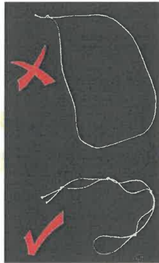
Figure 1. An example of correct “strops” to use to avoid seal entanglement.
