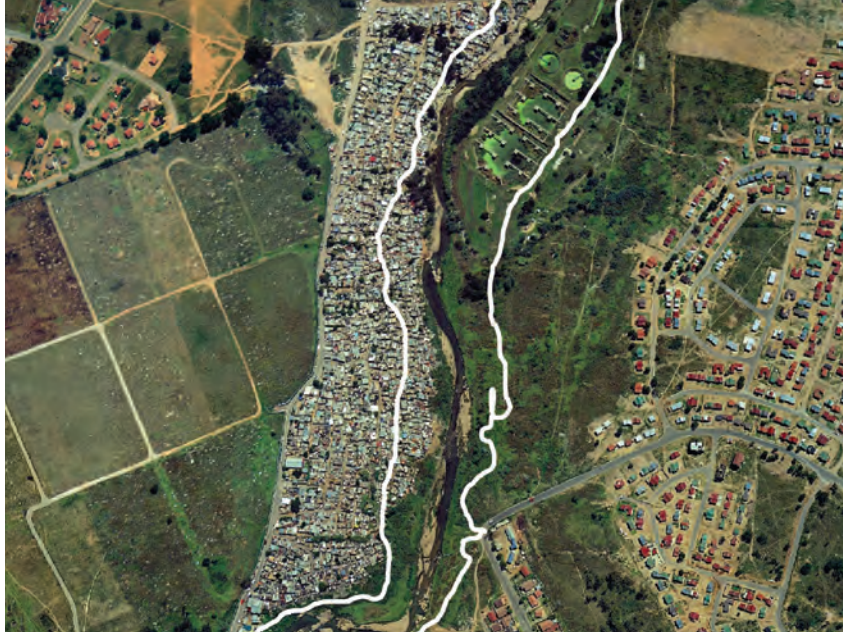
Map 10.6: Aerial photograph showing the proximity of informal settlements to the Jukskei River in Alexandra, Johannesburg. The 1:100 year floodline is indicated in white.
