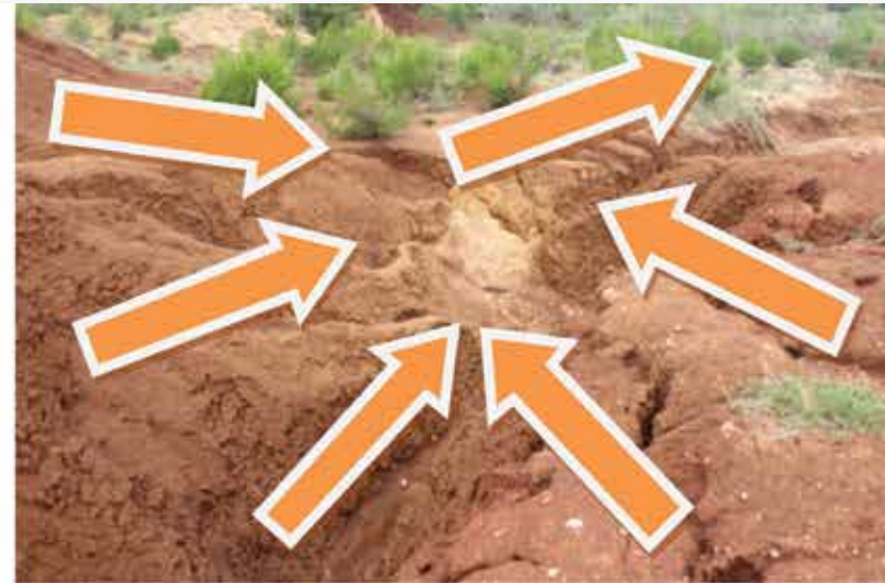
Picture 2 : Bathlabine brickyard factory area (owned and operated by Blue Platinum Ventures (Pty) Limited), which is approximately 100 meters from the nearby village, showing signs of sever soil erosion. This erosion is a result of the unlawful excavations undertaken in furtherance of a listed activity and negatively affects the nearby village especially during the rainy seasons.
