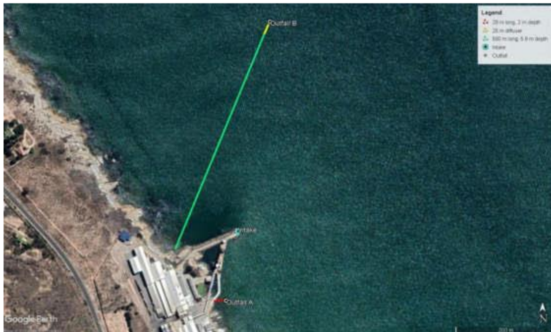
Figure 2: Aerial view of the two discharge points (Pipelines A and B) ( After the upgrade of the Pipelines )
