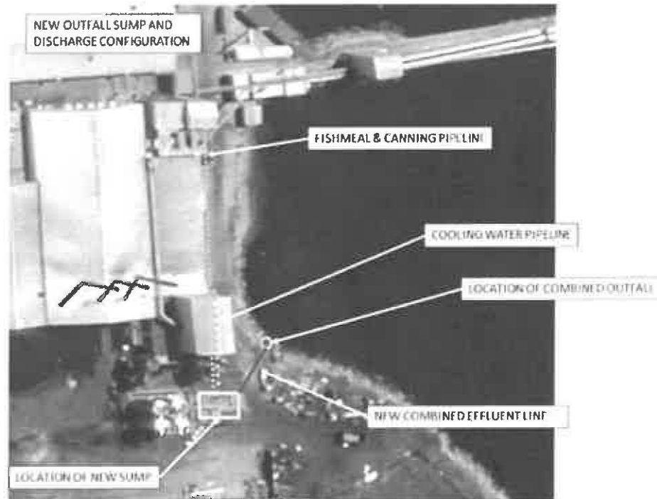
Figure 1: Aerial view of the Pioneer Fishing facility and the location of the effluent discharge point.
