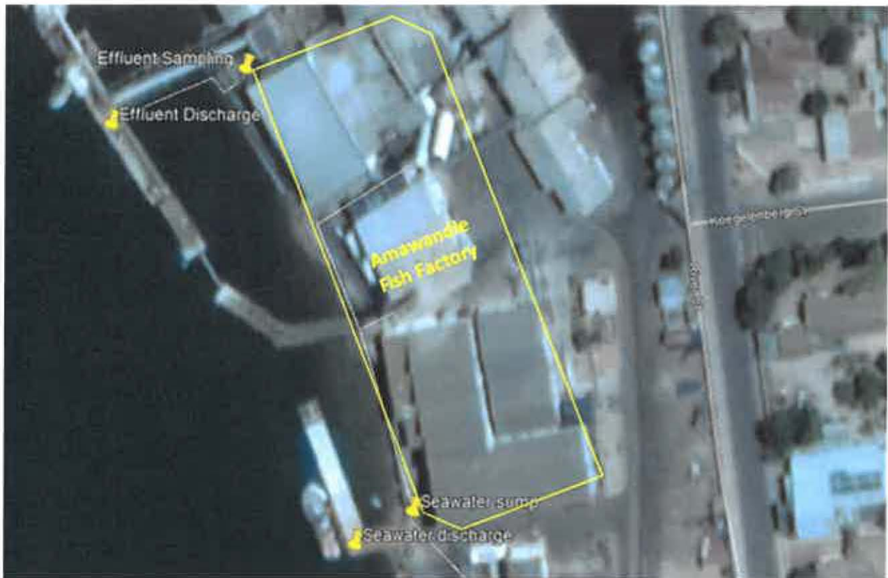
Figure 1: Aerial view showing Amawandle fish factory, effluent sampling locations and the two discharge points for the fish processing and seawater effluent streams
