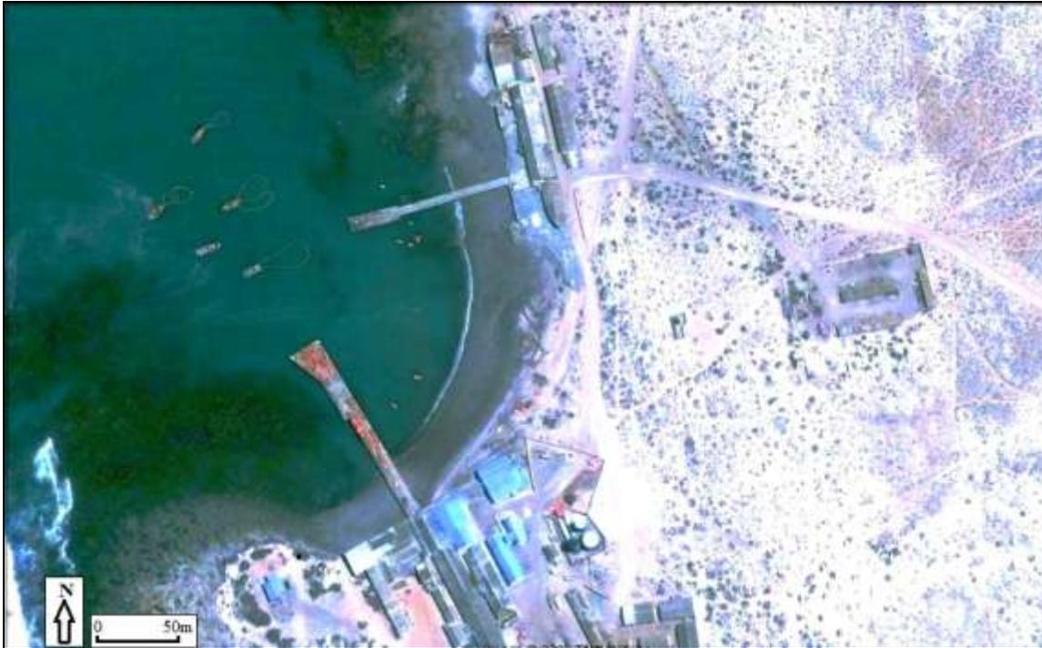
The harbour at Port Nolloth has become badly silted and now only the smallest of vessels can enter the harbour. The only vessels using Port Nolloth are fishing and pleasure craft and small vessels employed by the diamond mining industry.
