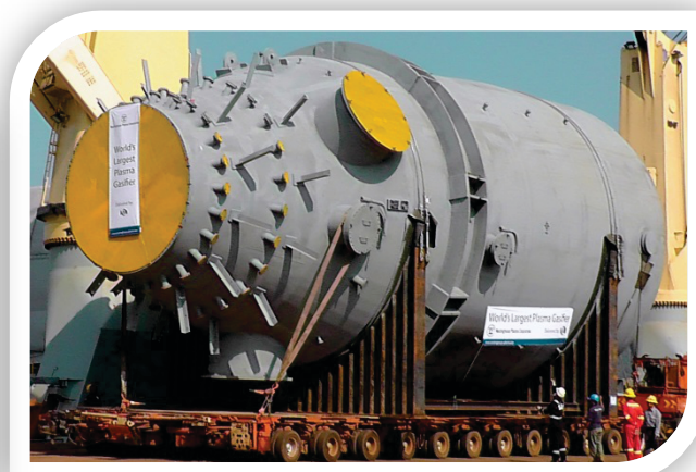
Figure 23: Demonstration plasma torches (image courtesy of AlterNRG); delivery of large (350k tonnes per annum) plasma gasifier in NE England (image
